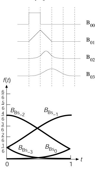
$$B_{00} = \begin{cases} B_{00} \\ B_{01} \end{cases} \qquad B_{k,0}(t) = \begin{cases} 1, & \text{if } t_k \le t < t_{k+1} \\ 0, & \text{otherwise} \end{cases}$$
