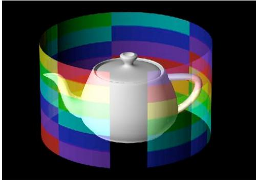
Given a point  $(x,y,z)$ , convert it to cylindrical coordinates  $(r, \theta, z)$  and use  $(\theta, z)$  as the 2D texture coordinates
